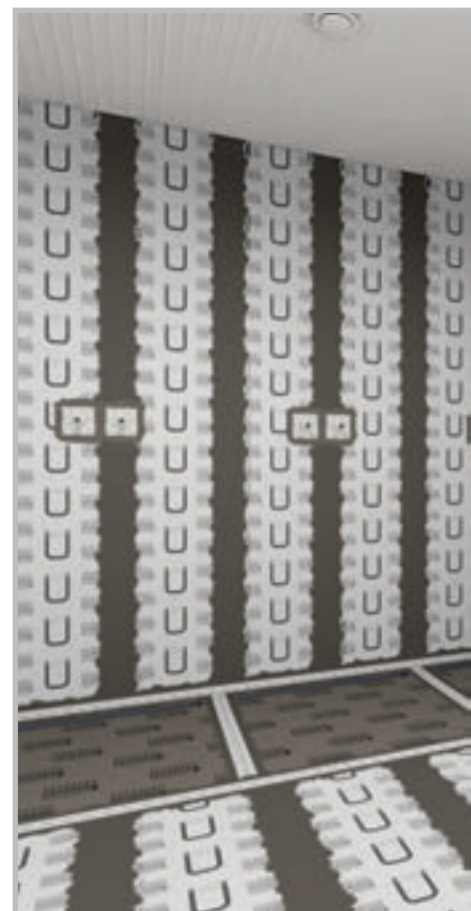
Shower area with sealing in a sheet form
